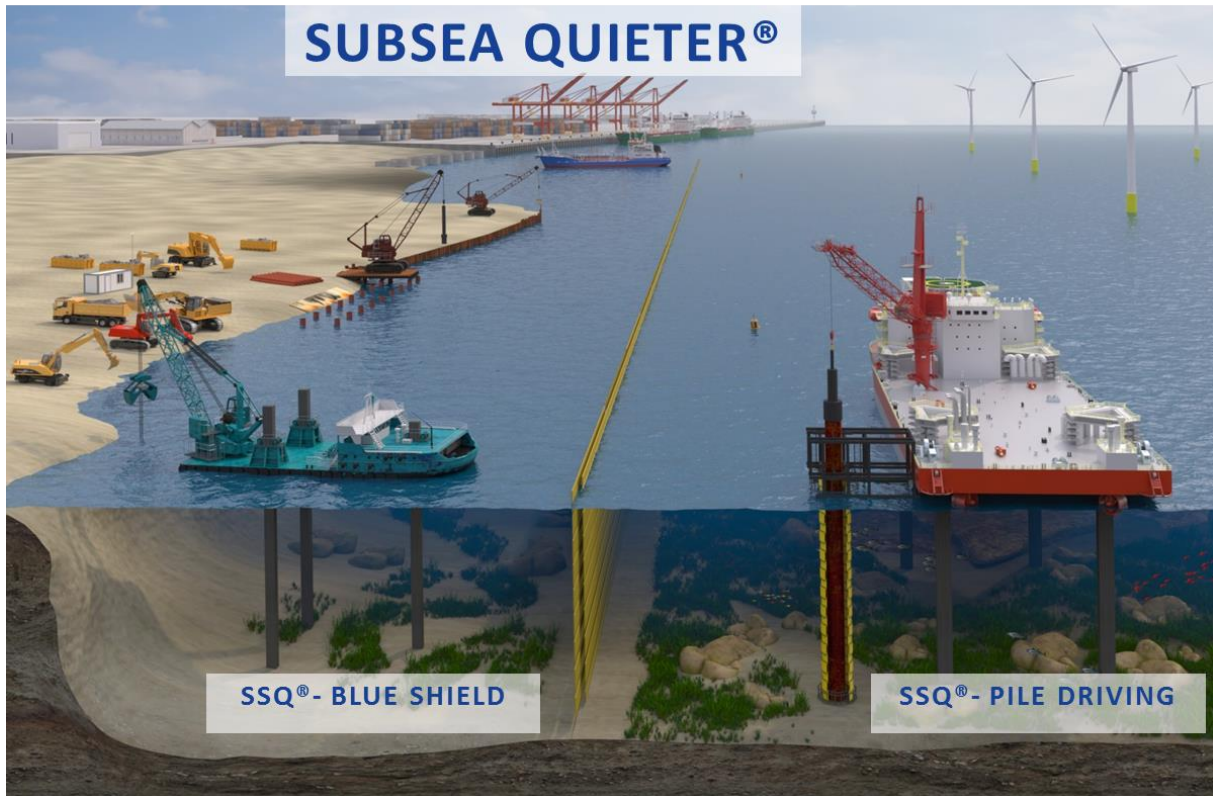
Image 1: Representation of the two types of the SubSea Quieter. Source: Greenov®
